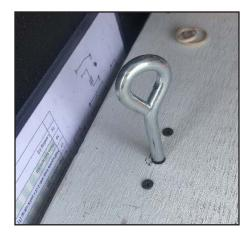
Next you will need a stop to hold the top sheet in position when driving. I cut two pieces of 2x4 wood, one for each side, that matched the spacing between the top and bottom sheets. These I screwed to the bottom sheet about 4" from the table end and 3" from each side. Then I drilled a ½" hole through the two sheets and wood blocks. Then used a long bolt as a pin to lock the top sheet in place.
