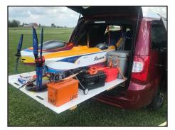
To use the slide, pull the two pins and pull the top sheet out about 5/8 of way, just enough so you can fold the table leg down and clear the van. (Mark the position so it is easily repeatable.) The side angles will hold the sheet up while you unfold the dining leg. Then slightly lift the top sheet and pull it out the rest of way, leaving about 6" left in the tracks.
