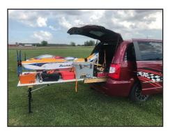
If you want even more storage, you can also use PVC tubing and build a frame that rests on top of the angle brackets. Lay some  $1 \frac{1}{2}$ " insulating foam on top of the frame to create a shelf. With this shelf in place I have carried more than a dozen planes to an event including the 35%, a 25%, a Radian Pro, and the equipment needed for a weekend.
